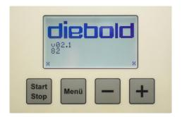
After switching on the device the Software version (in picture "v02.1") and the Number of shrink cycles (in picture "82") will be displayed for approx. 3 seconds.
